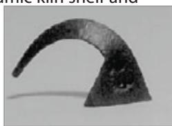
*A self-supporting cone fired to maturity (do not be concerned if the tip is slightly higher or lower than shown).*
