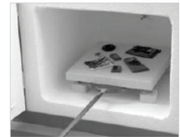
**Please Note:** For safest cooling, leave the piece inside the kiln until the kiln cools to room temperature.
